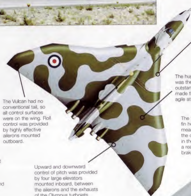
The Vulcan's unique delta wing made it highly manoeuvrable for such a large machine.
